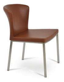
Capri Metal is a contemporary dining chair with a comfortable upholstered seat and backrest on chrome plated steel legs. The seat has a steel structure with "S" shape springs for extra flexibility and strength. Capri Metal is also available in a lower seat (stool seat) upon desire. This steel frame is moulded by injecting polyurethane foam. Capri Metal is suitable for both residential and commercial use.
