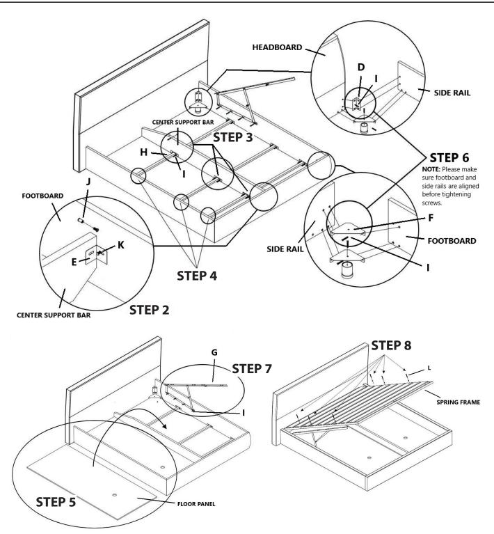
**CAUTION:** To avoid any damage on the hydraulics and bed, please do not pull down the spring frame without putting the mattress on first as the added weight will help alleviate the motion and mechanism on the hydraulics. Any damages caused by forcefully pulling down the spring frame by itself will void the warranty. Maximum weight capacity is 220 lbs.
