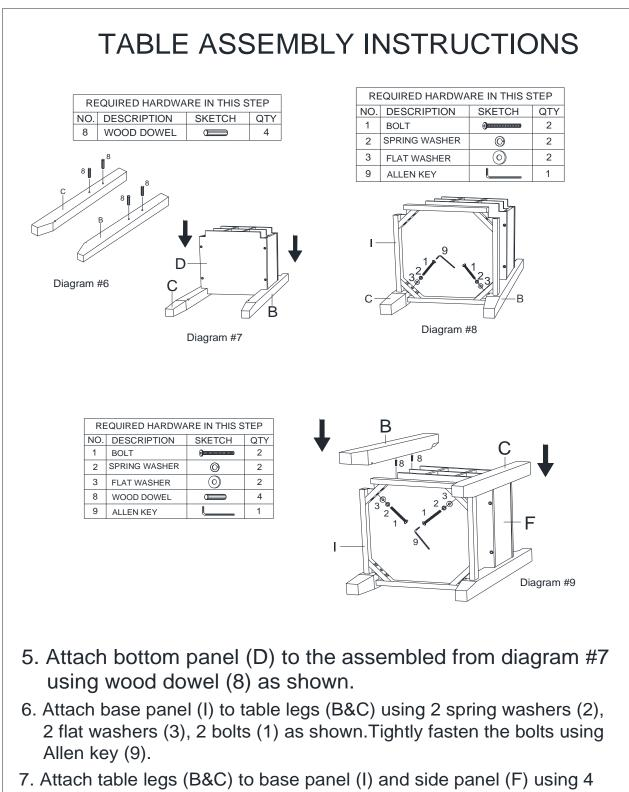
Attach table legs (B&C) to base panel (I) and side panel (F) using 4 wood dowel (8), 2 spring washers (2), 2 flat washers (3) and 2 bolts (1) as shown. Tightly fasten the bolts using Allen key (9).
