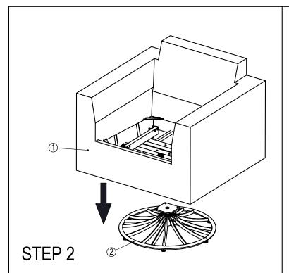
ALIGN THE HOLES OF BODY AND BASE SWIVEL ROCKER UNTIL ALL HOLES ARE CENTERED
