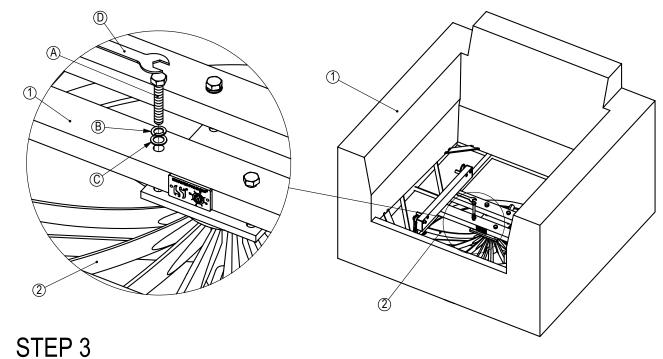
AFTER THE BODY AND BASE HOLES ARE CENTERED THREAD THE BOLTS ONE BY ONE BEFORE FULLY TIGHTENING THEM ALL
