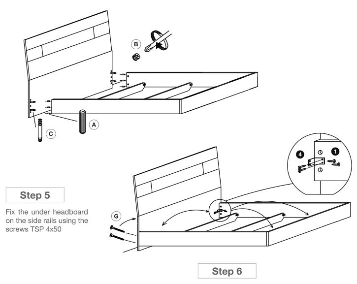
Fit the iron corner on the side rails and to the under headboard, using the screws TSP 4x16
