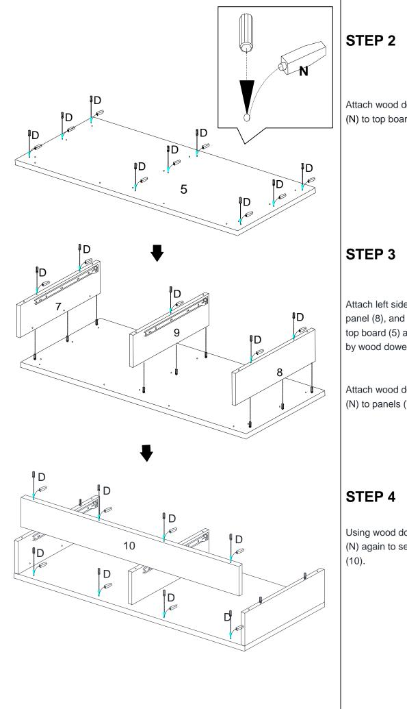
Attach wood dowels (D) with Glue (N) to top board (5) as shown.
