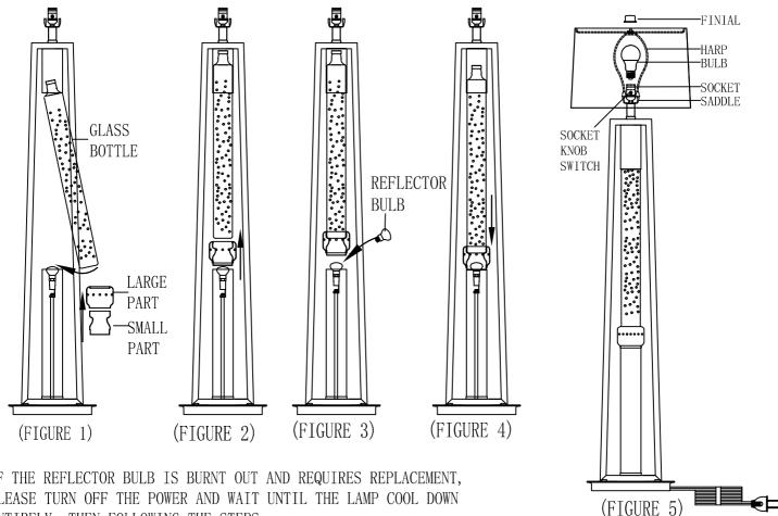
IF THE REFLECTOR BULB IS BURNT OUT AND REQUIRES REPLACEMENT, PLEASE TURN OFF THE POWER AND WAIT UNTIL THE LAMP COOL DOWN ENTIRELY, THEN FOLLOWING THE STEPS.
