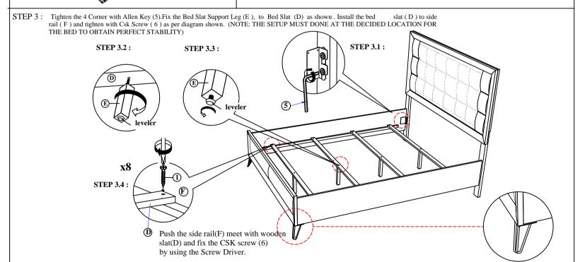
NOTE: MUST TIGHTEN SCREWS PERIODCALLY WITH USE SCREW WILL BECOME LOOSE CHECK TIGHTNESS OF ALL SCREW EVERY 6-8 WEEKS.
