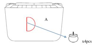
STEP #2 Align the legs to the bottom seat of the pre-drilled holes, rotate to tighten the legs.
