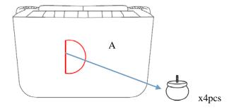
STEP #2 Align the legs to the bottom seat of the pre-drilled holes, rotate to tighten the legs.
