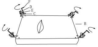
Step 4. Attach the back rest onto the back rail Velcro and fix in the position properly.
