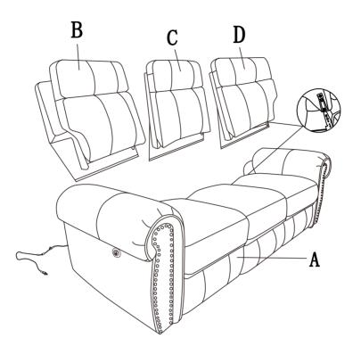
STEP#3 Attach Plug with Wire(E) to the Power Switch
