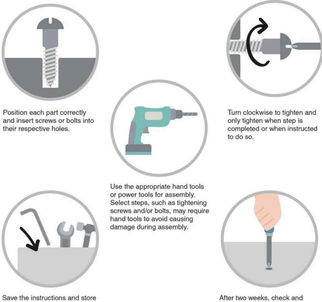
Save the instructions and store any supplied tools for later maintenance. After two weeks, check and tighten any loose hardware and repeat again every six months thereafter.
