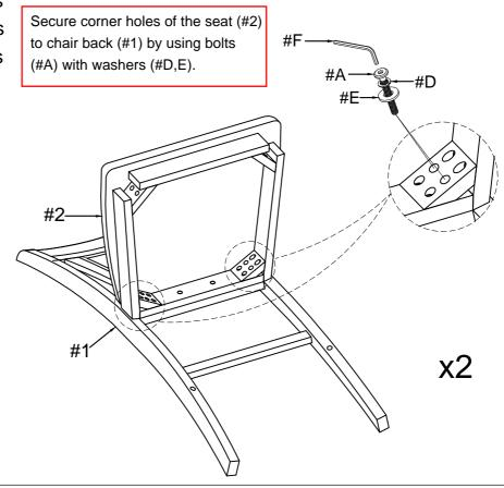
Part #6 x1pc Align stretchers (#6,7) to the chair back Part #7 x1pc legs. x2 #F Align front legs (#3,4) to the #D Part #3 x1pc stretchers (#5,6,7) and seat (#2), Part #4 x1pc then secure front legs (#3,4) to seat (#2) by using bolts (#B) with Part #5 x1pc washers (#D,E). Hardware #B x4pcs Hardware #D x4pcs Hardware #E x4pcs #5 x2
