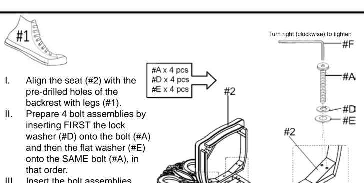
III. Insert the bolt assemblies through the pre-drilled holes in the corners of the seat (#2) and secure those bolts using the Allen wrench (#F) to lock them in with the backrest with legs (#1).
