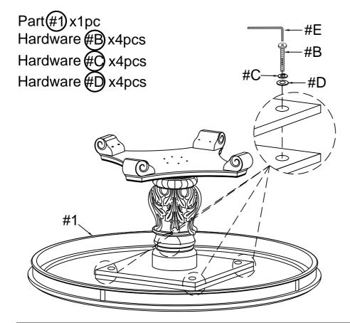
Align table base to the table top (#1), then secure by using bolts (#B) with washers (#C,D).
