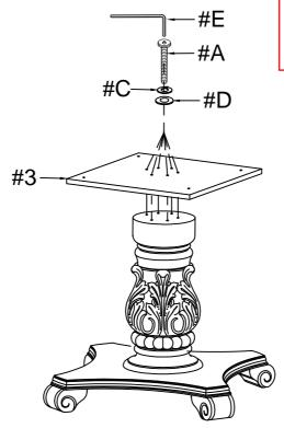
Align table top base (#3) to the pedestal, then secure by using bolts (#A) with washers (#C,D).
