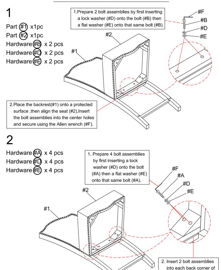
the seat (#2) and secure using the Allen wrench.
